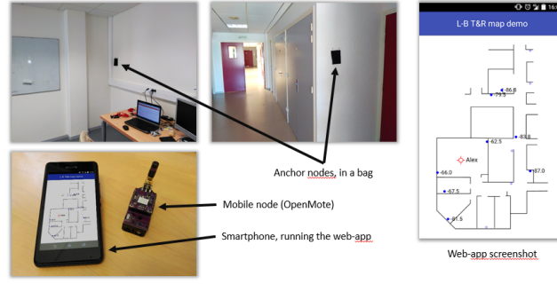
Figure 3.8: Deployment of the radio localization demonstrator in an indoor environment
